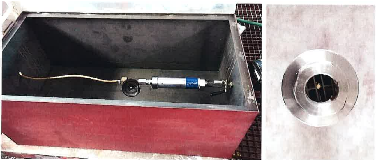
Picture 2 IPS BlueLine in the test cabinet and during distance measurement.
